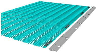
The repair kit uses (4) reinforcing plates for each connection. These plates are centered on the hole/bolt locations 1, 3, 6 and 8. Line one of the replacement extrusions up with the mat and mark the bolt locations on the mat.
