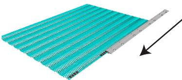
Slide the extrusion piece onto the mat from one side, insuring the reinforcing plates remain in place. The extrusion is slightly narrower than the mat, so center the extrusion on the mat
