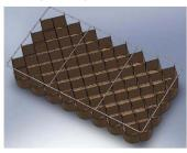
Pull out next cell unit and fit frame. Place on top of filled bottom unit.
